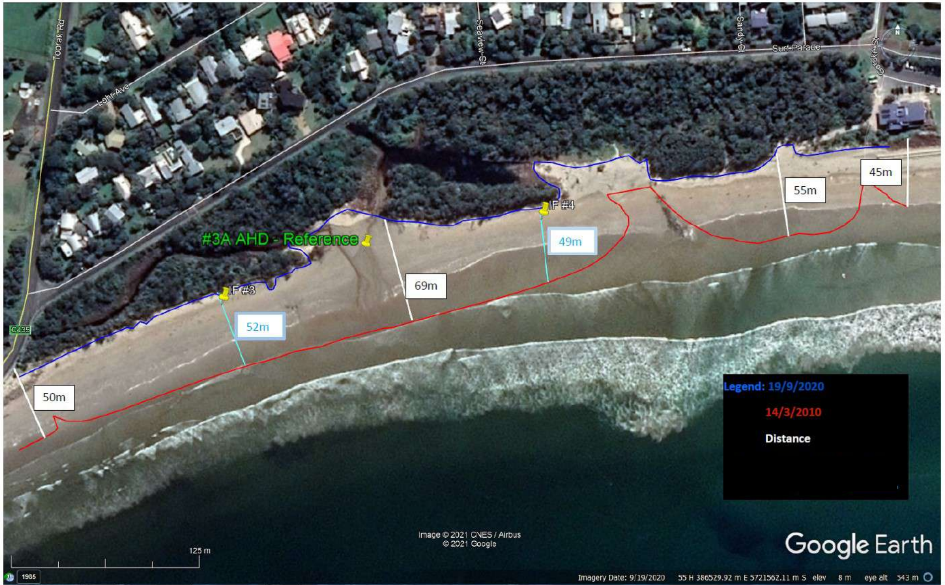
Figure 6 Annotated Google Earth image of the Wreck Creek coastline (SLC to Eastern end of Rock Wall) showing Dune Loss from 14/3/2010 to 19/9/2020
