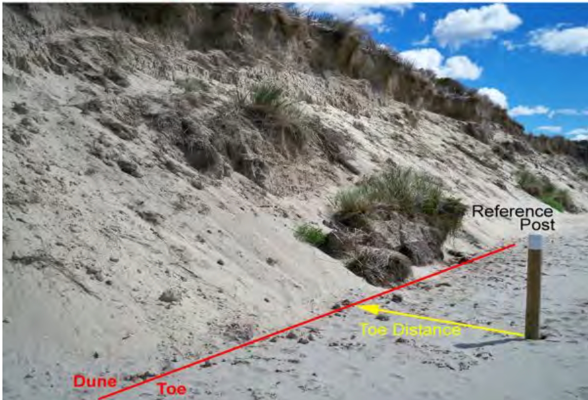
Fig. 31: Measuring dune recession at East Beach, Port Fairy. Courtesy: Port Fairy Coastal Group.
