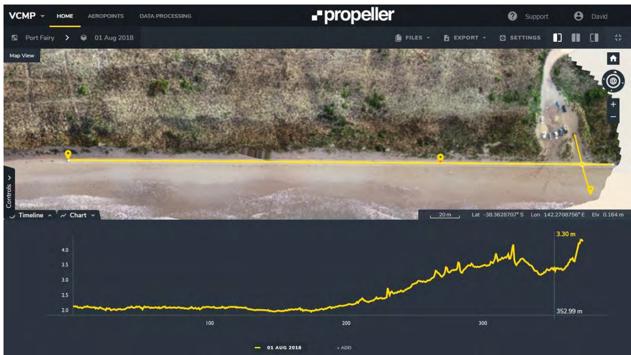
Fig. 35: Drone monitoring data showing a longitudinal cross-section at East Beach, Port Fairy. Courtesy: Deakin University, Warrnambool.
