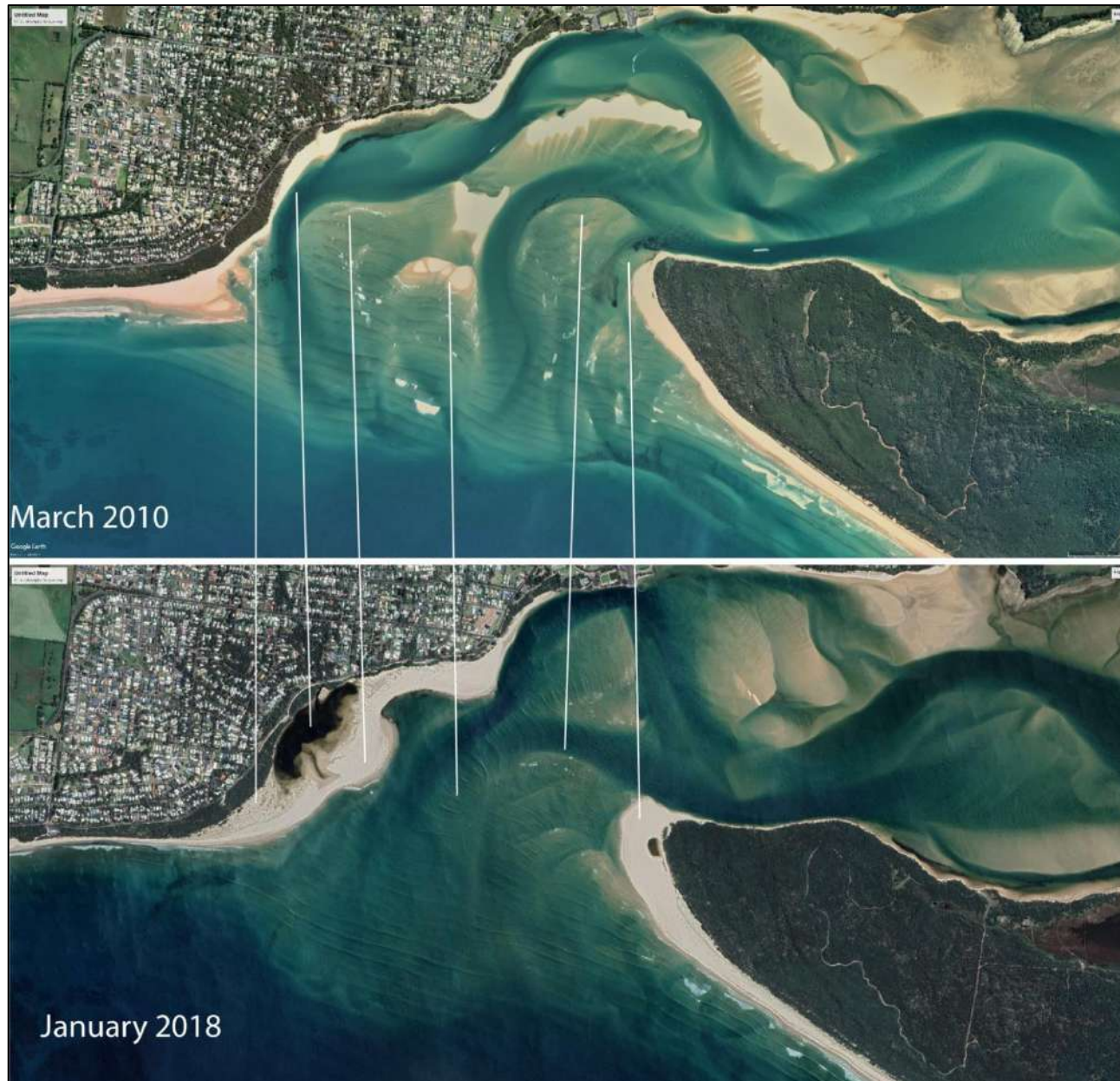
Figure 25. Ebb tide delta and channels 2010 and 2018. Multiple ebb-tide channels in 2010 are replaced by a single ebb-flood channel in 2018. Lines join same point on both images (Google Earth)
